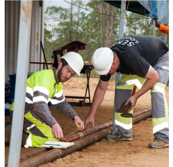
SEMM Logging, on-site core assessment (2017)
